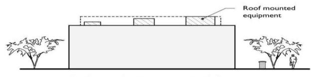
Roof mounted equipment screening shall be an encompassing monolithic unit and shall be the same height as the equipment.
