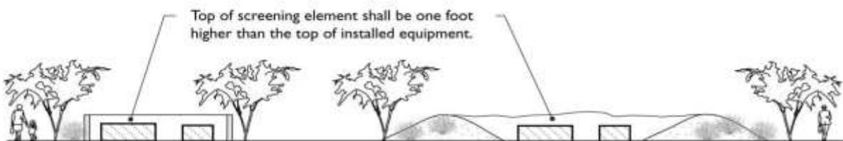
**Figure 18.80.110.A.2. Screening of Ground-Mounted Equipment**
