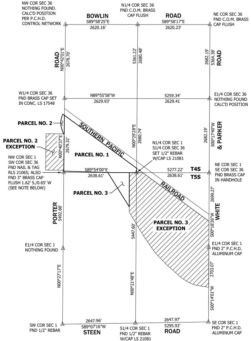
NOTE: The found brass cap flush appears to have been set by Edward Vincent, R.L.S. 17548 per Record of Survey, Fee No. 2010-116895 but was not accepted as the section corner by this surveyor.
