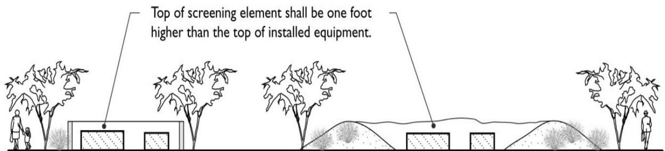
Figure 18.80.110.A.2. Screening of Ground-Mounted Equipment
