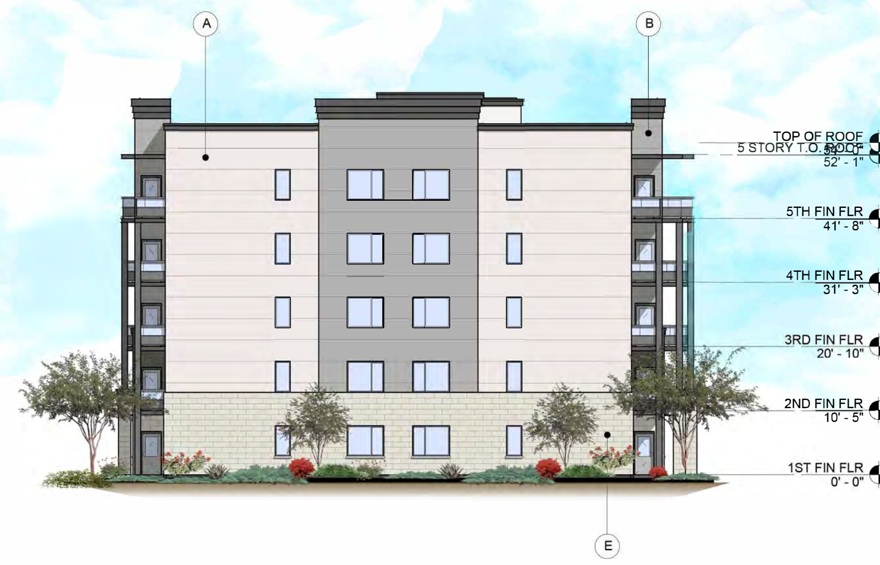
BLDG TYPE 1 - LEFT ELEVATION
