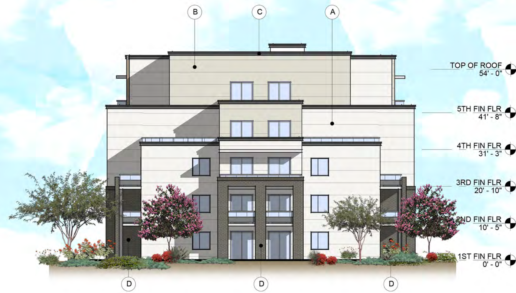
3 BLDG TYPE 4 - LEFT ELEVATION 1/16" = 1'-0"
