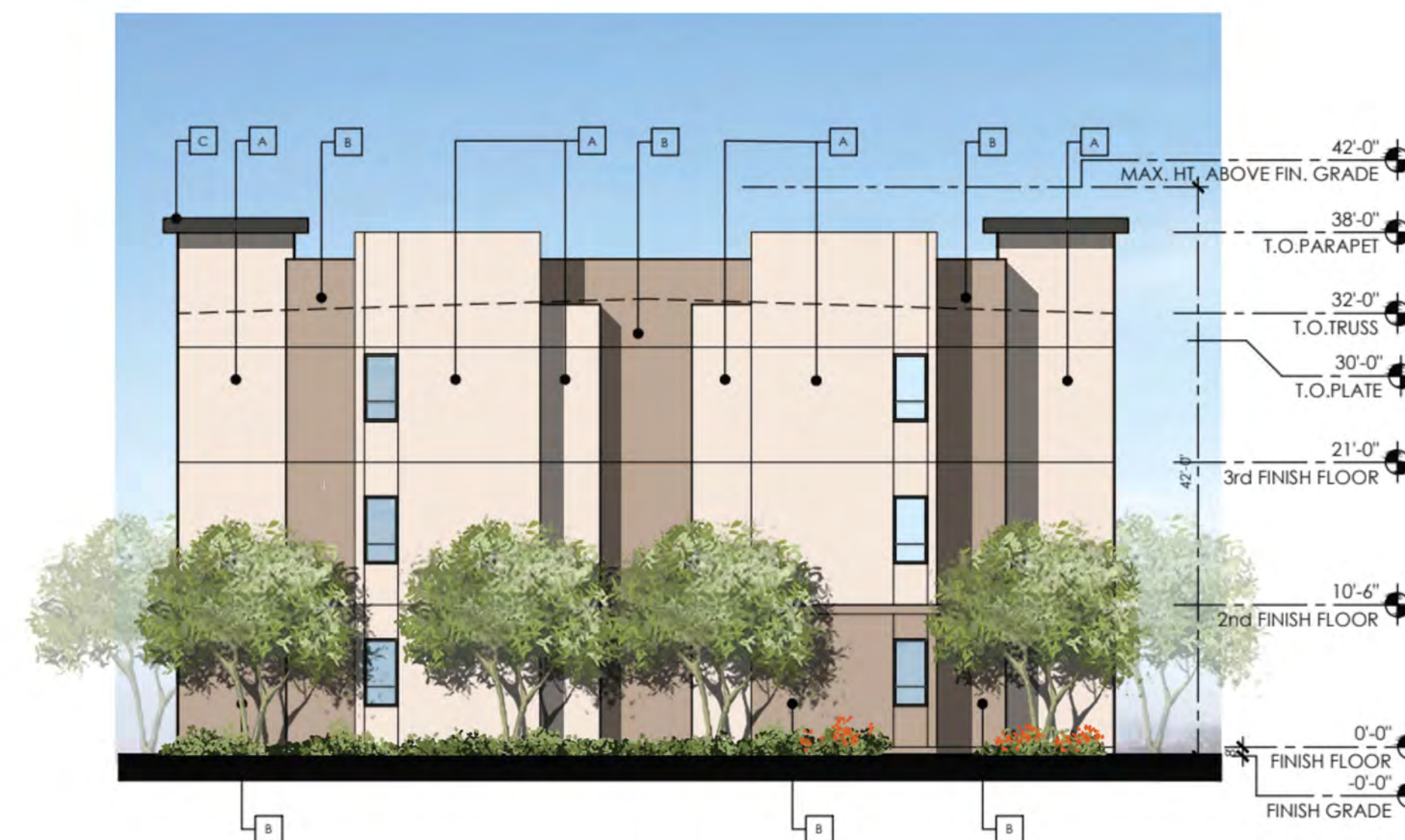
BUILDING TYPE 2 RIGHT ELEVATION
