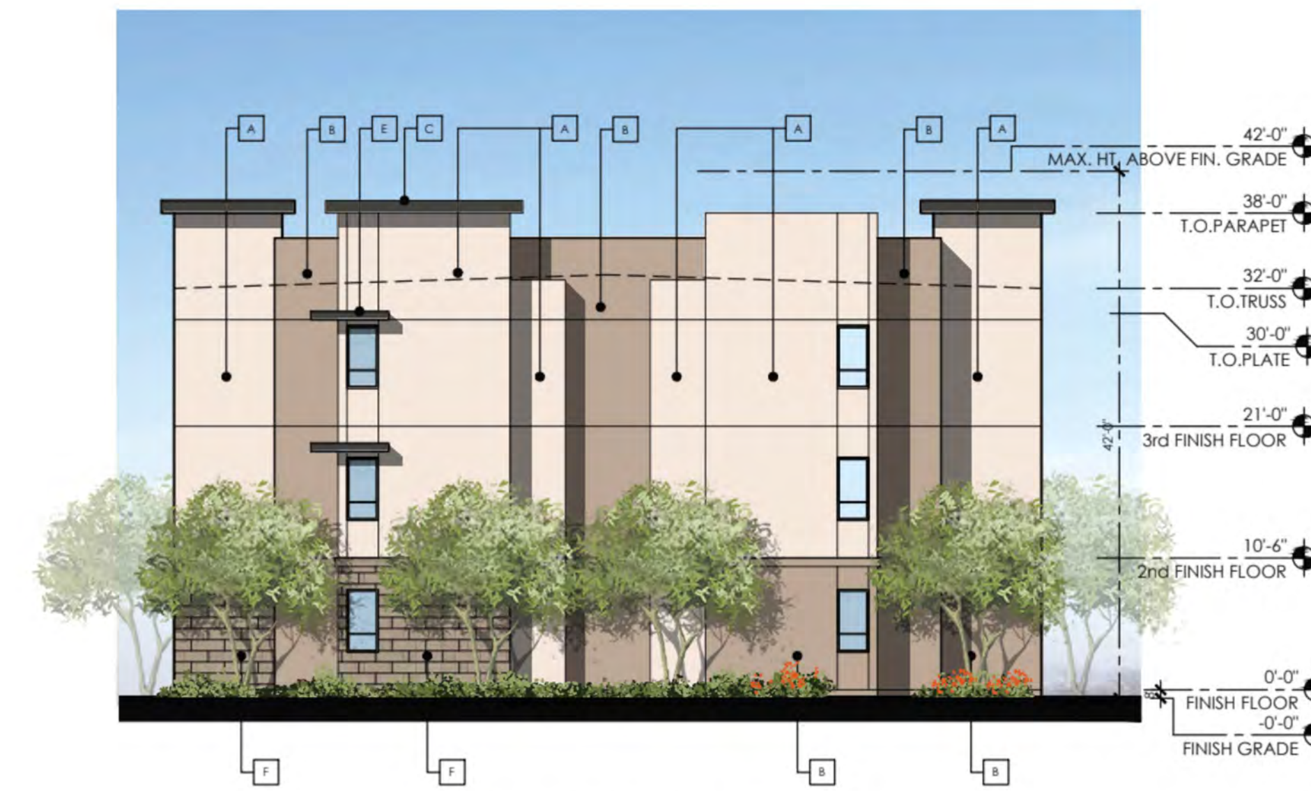
BUILDING TYPE 1C RIGHT ELEVATION
