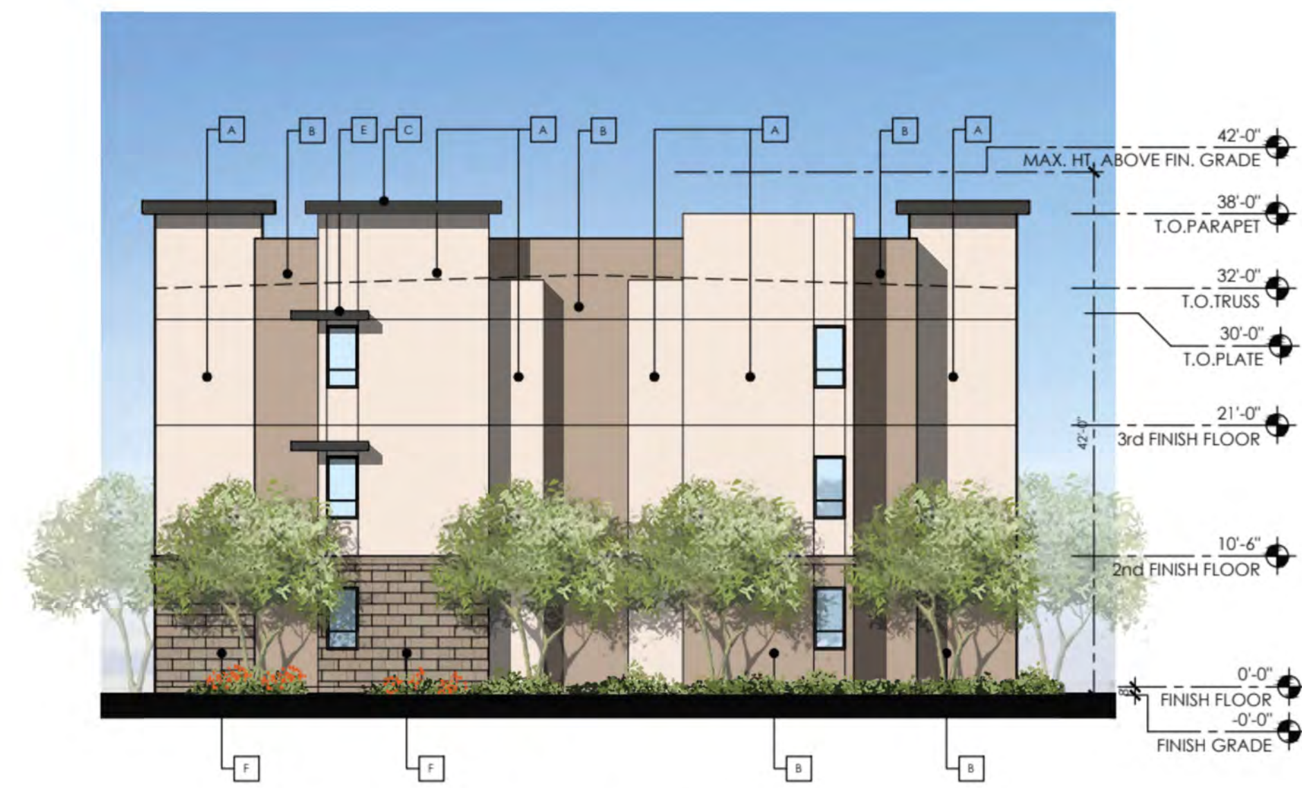
BUILDING TYPE 1B LEFT ELEVATION
