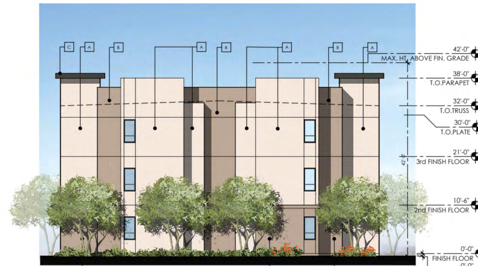
BUILDING TYPE 2 RIGHT ELEVATION
