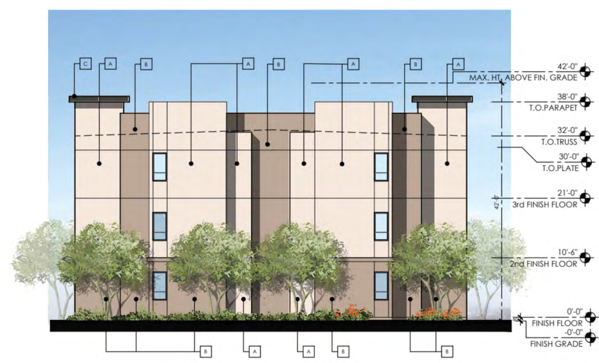
BUILDING TYPE 1A RIGHT ELEVATION
