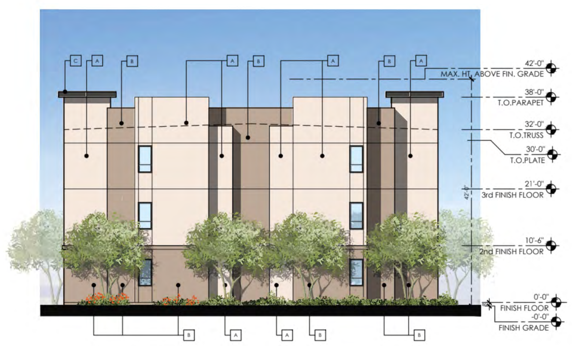
BUILDING TYPE 1A LEFT ELEVATION
