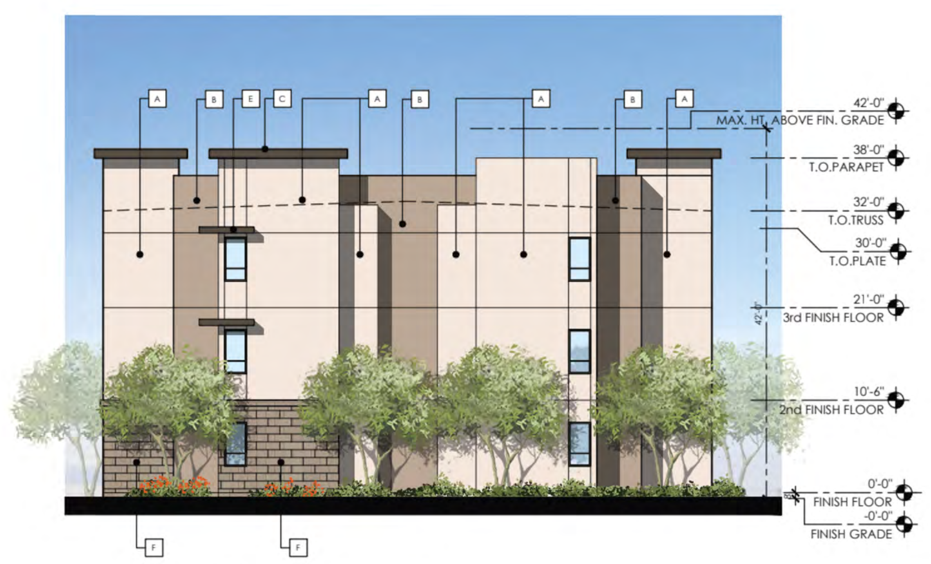
BUILDING TYPE 1 LEFT ELEVATION
