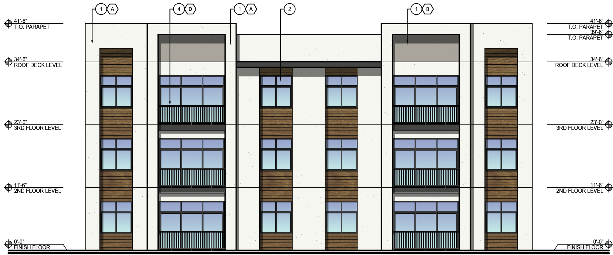
3 ELEVATION 3 - BUILDINGS 5 & 6 - TYPICAL 3/32" = 1'-0"
