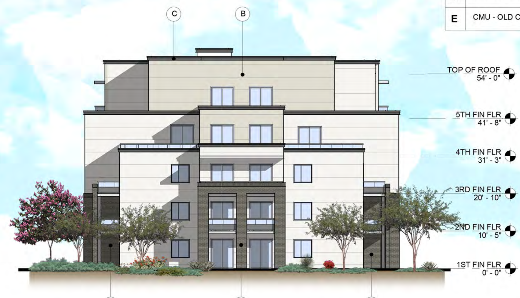
4 BLDG TYPE 4 - RIGHT ELEVATION 1/16" = 1'-0"
