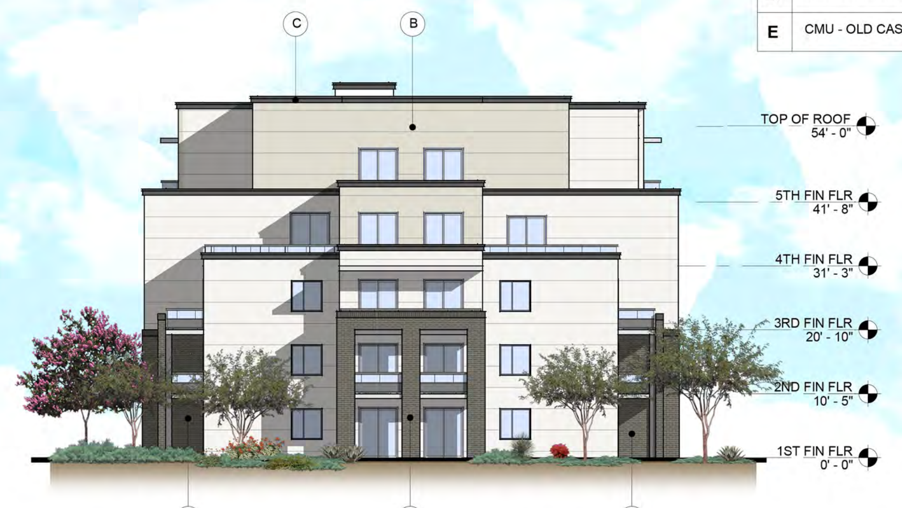
4 BLDG TYPE 4 - RIGHT ELEVATION 1/16" = 1'-0"
