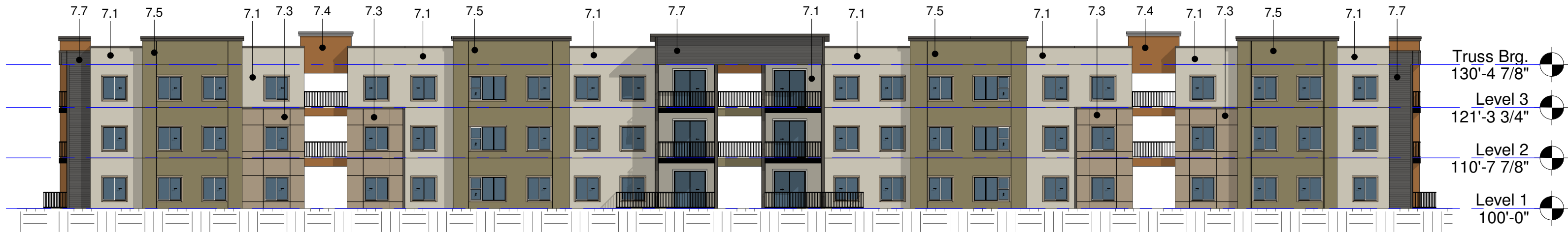
3 Exterior Elevation - Back 1" = 20'-0"
