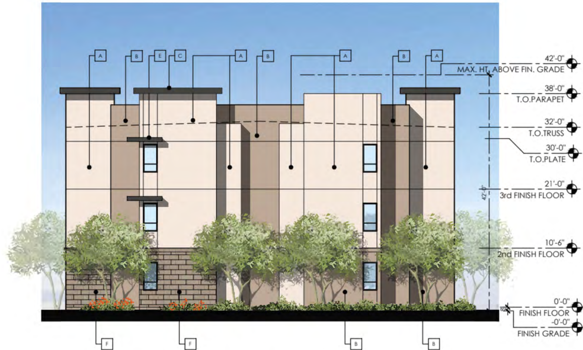
BUILDING TYPE 1B LEFT ELEVATION
