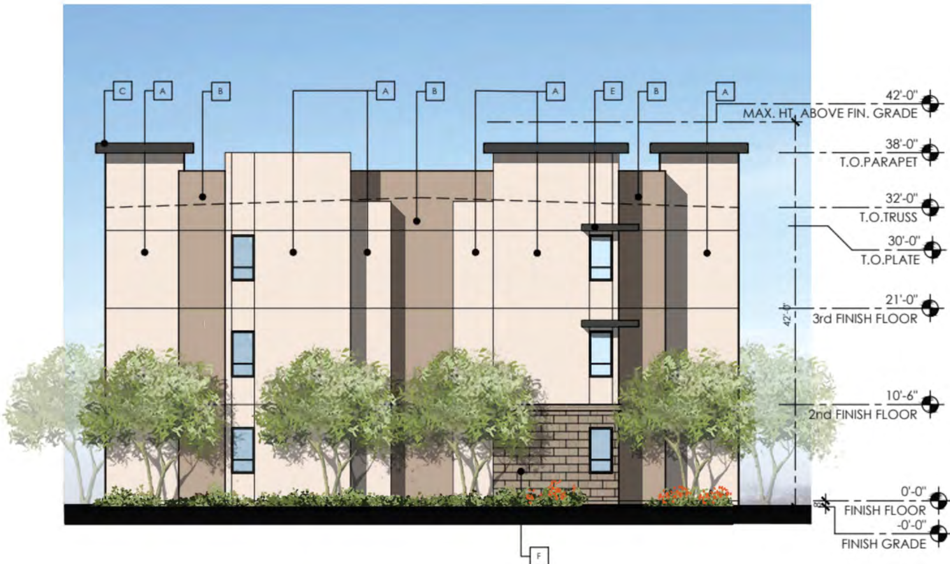
BUILDING TYPE 1D RIGHT ELEVATION
