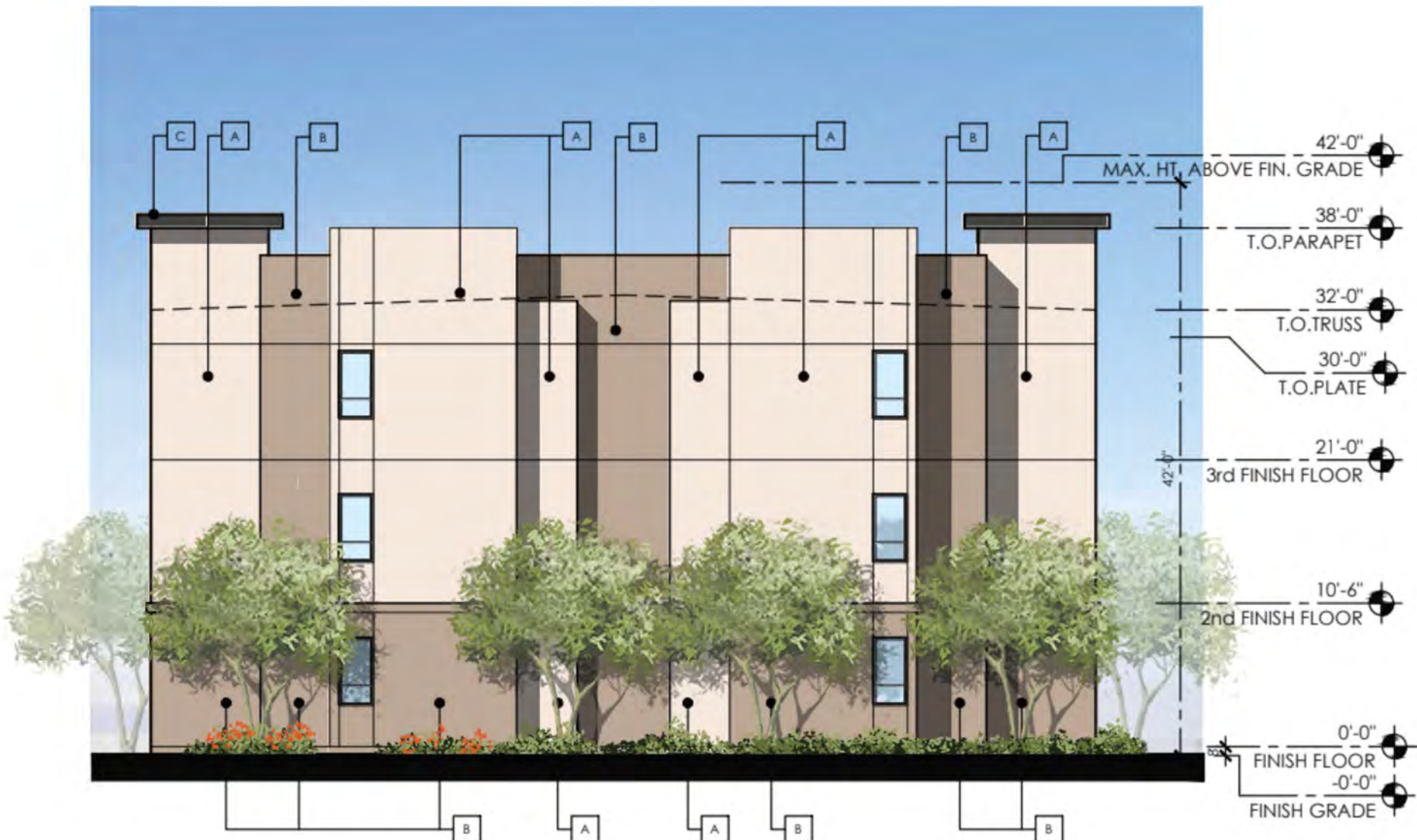
BUILDING TYPE 1A LEFT ELEVATION
