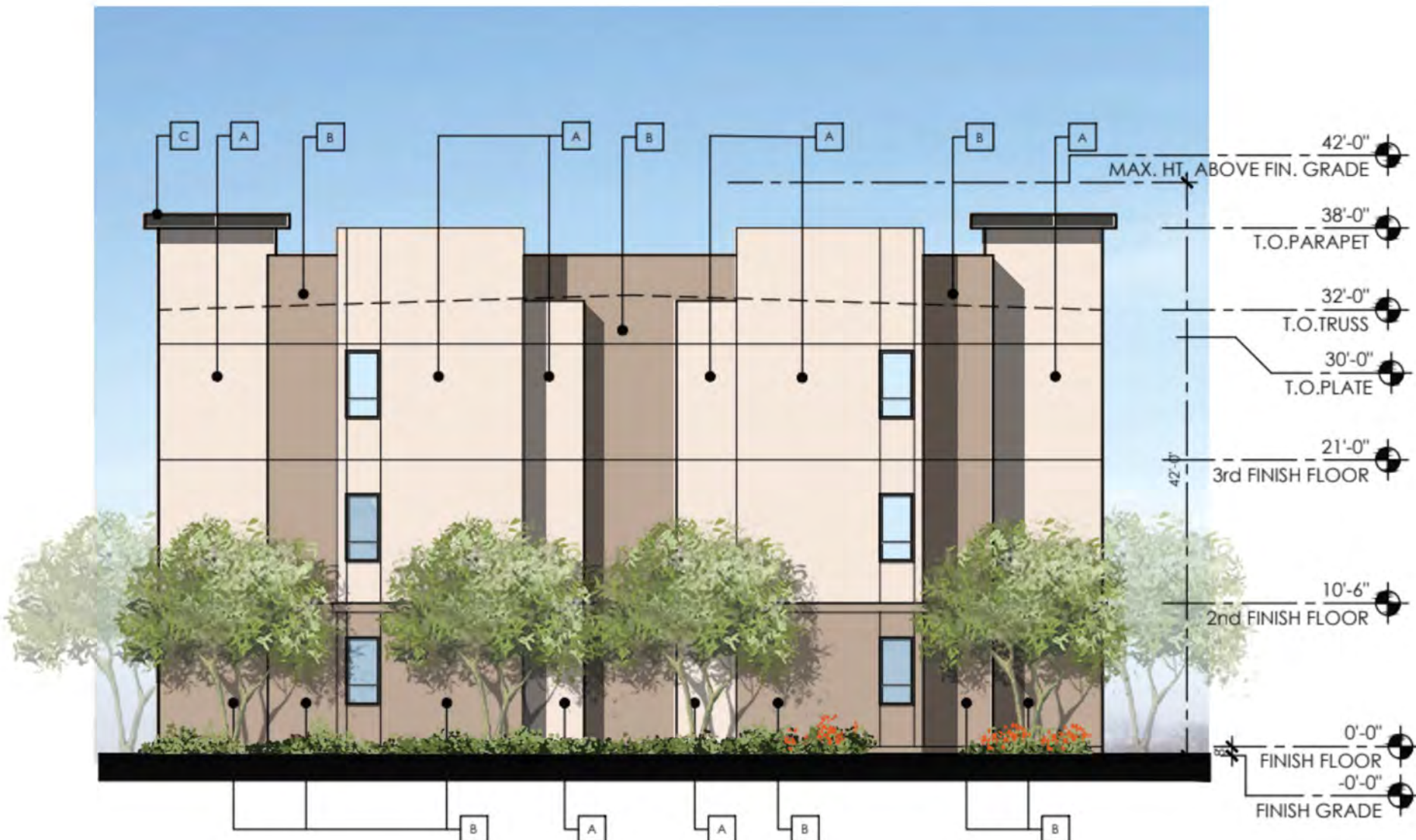
BUILDING TYPE 1A RIGHT ELEVATION
