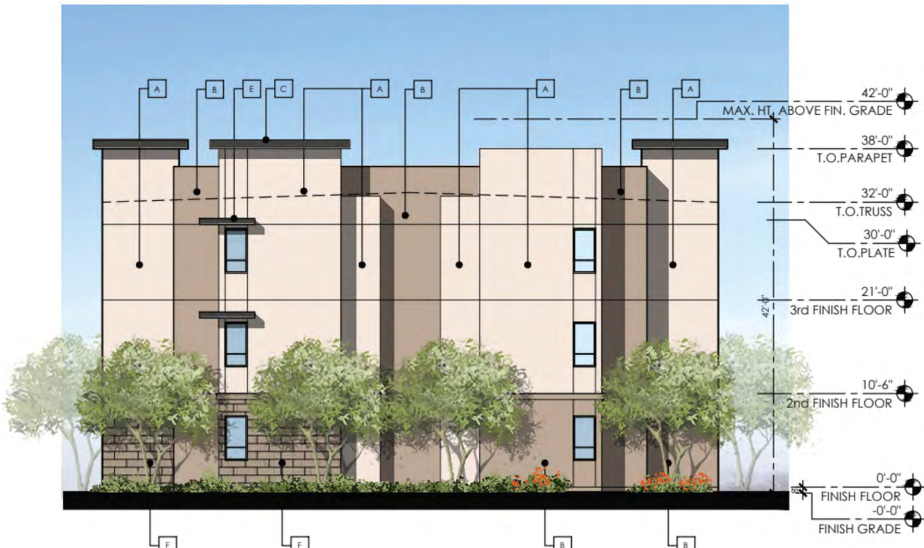
BUILDING TYPE 1C RIGHT ELEVATION
