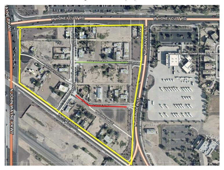
Scope of Work: Full roadway width pavement, installation of concrete roll curb, gutter, sidewalks, and ADA compliant sidewalk ramps. Installation of a 30' dusk-to-dawn street light.
