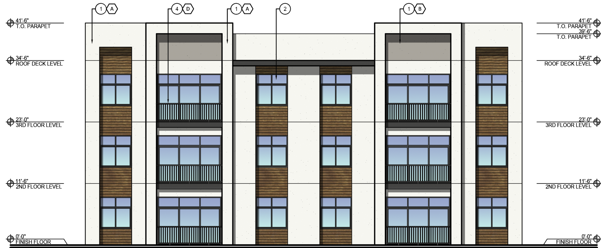
3 ELEVATION 3 - BUILDINGS 5 & 6 - TYPICAL 3/32" = 1'-0"
