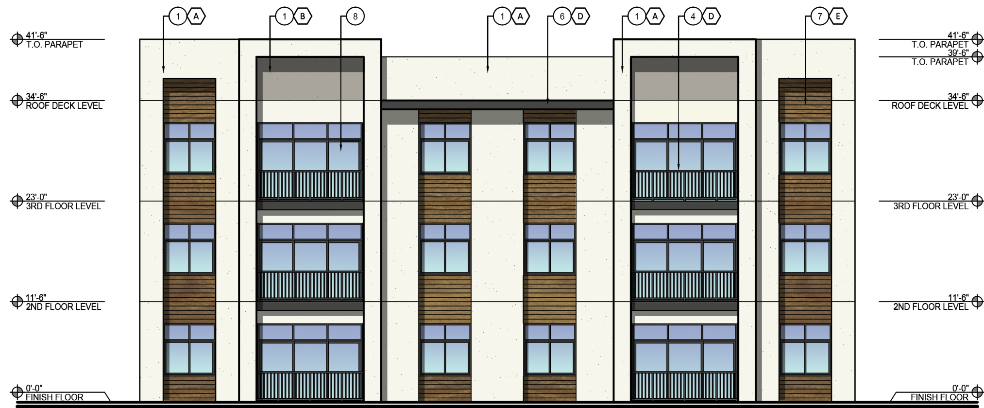
3 ELEVATION 3 - BUILDINGS 1, 2 & 3 - TYPICAL 3/32" = 1'-0"
