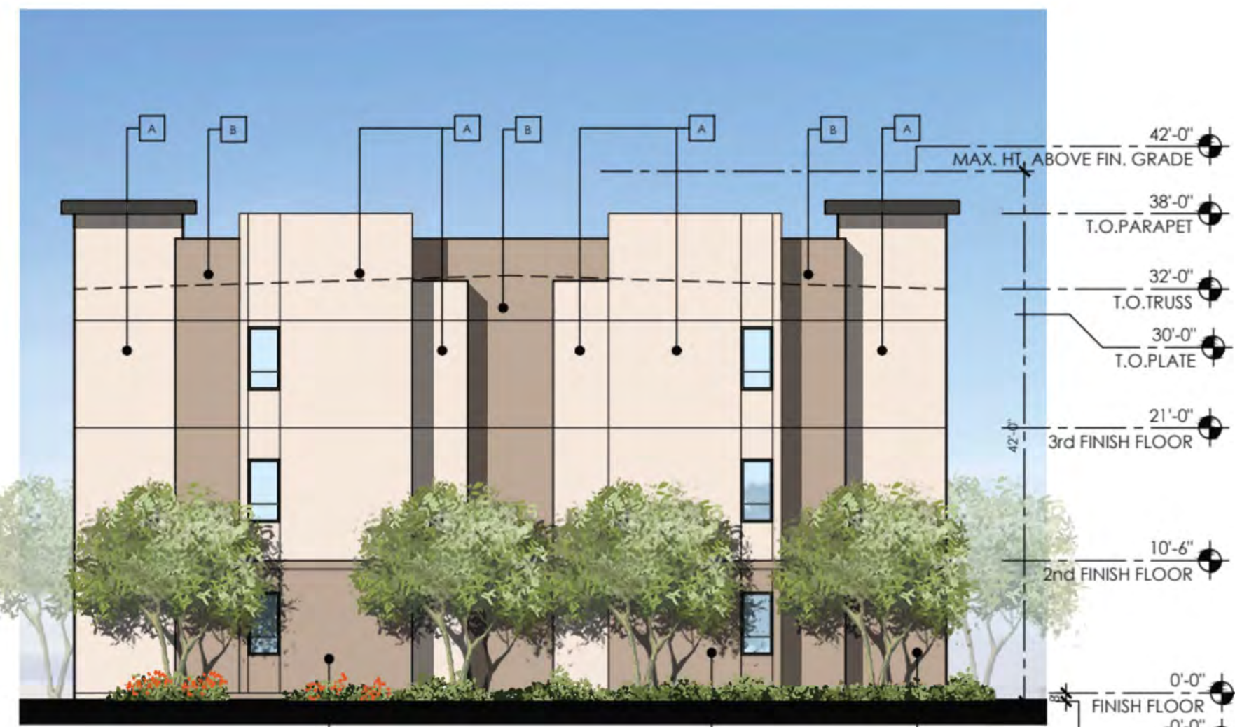
BUILDING TYPE 2 LEFT ELEVATION
