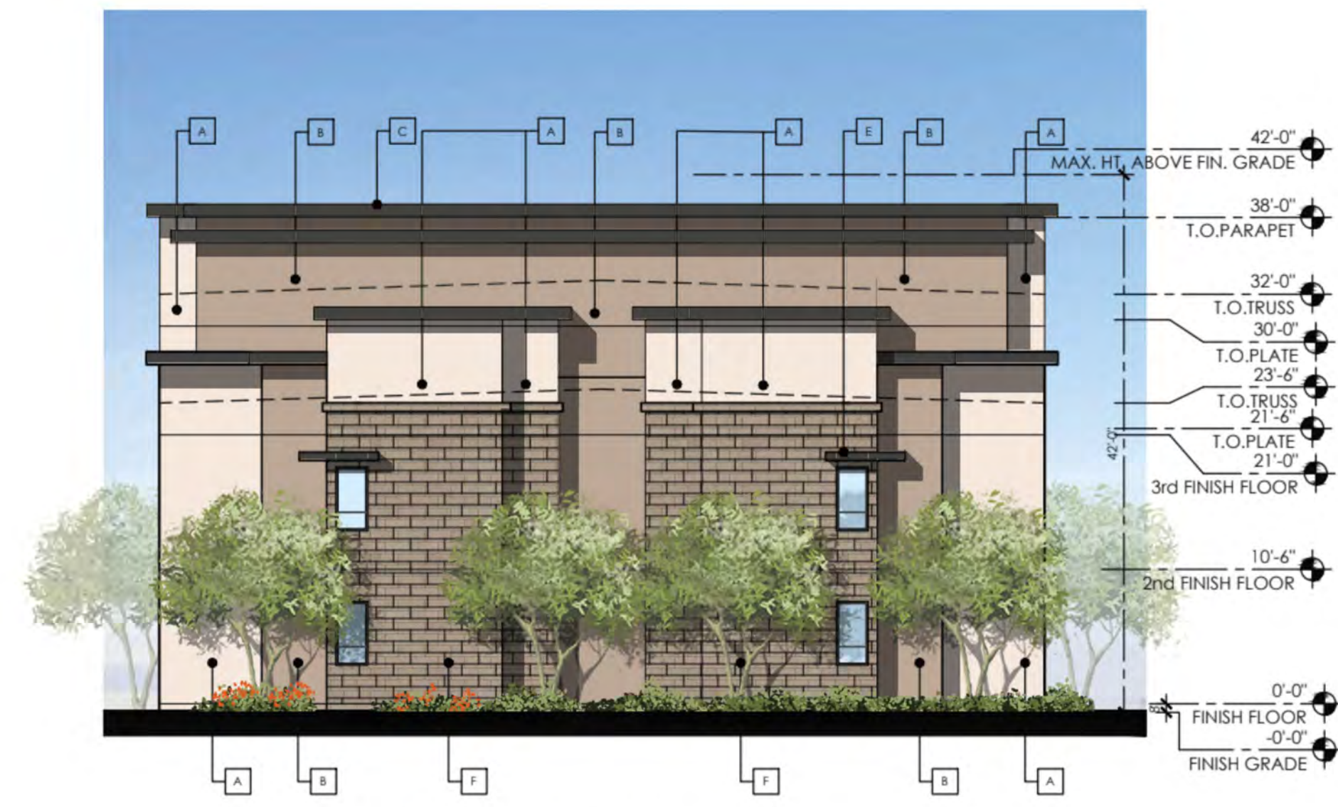
BUILDING TYPE 1C LEFT ELEVATION
