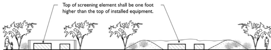
FIGURE 401.11.A.2: SCREENING OF GROUND-MOUNTED EQUIPMENT
