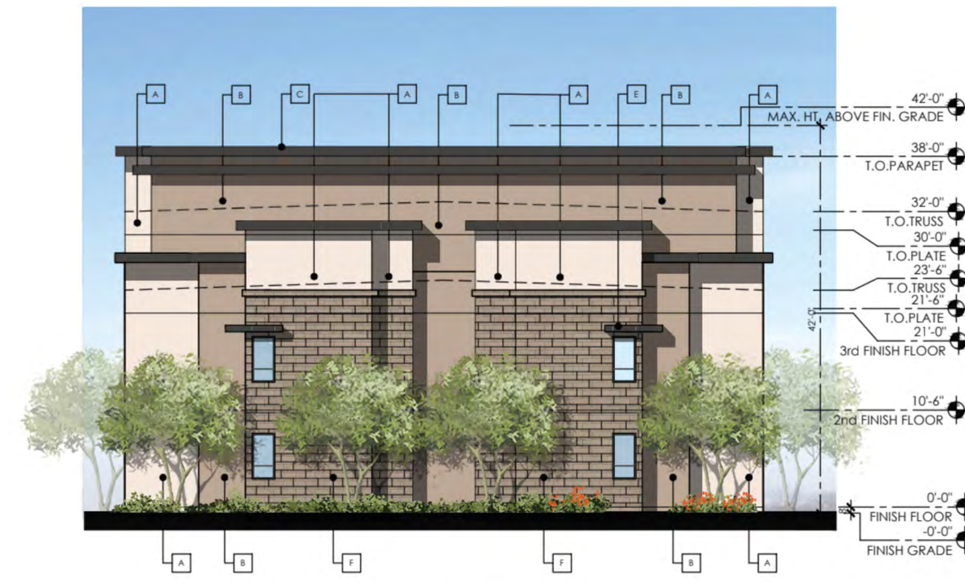
BUILDING TYPE 1B RIGHT ELEVATION
