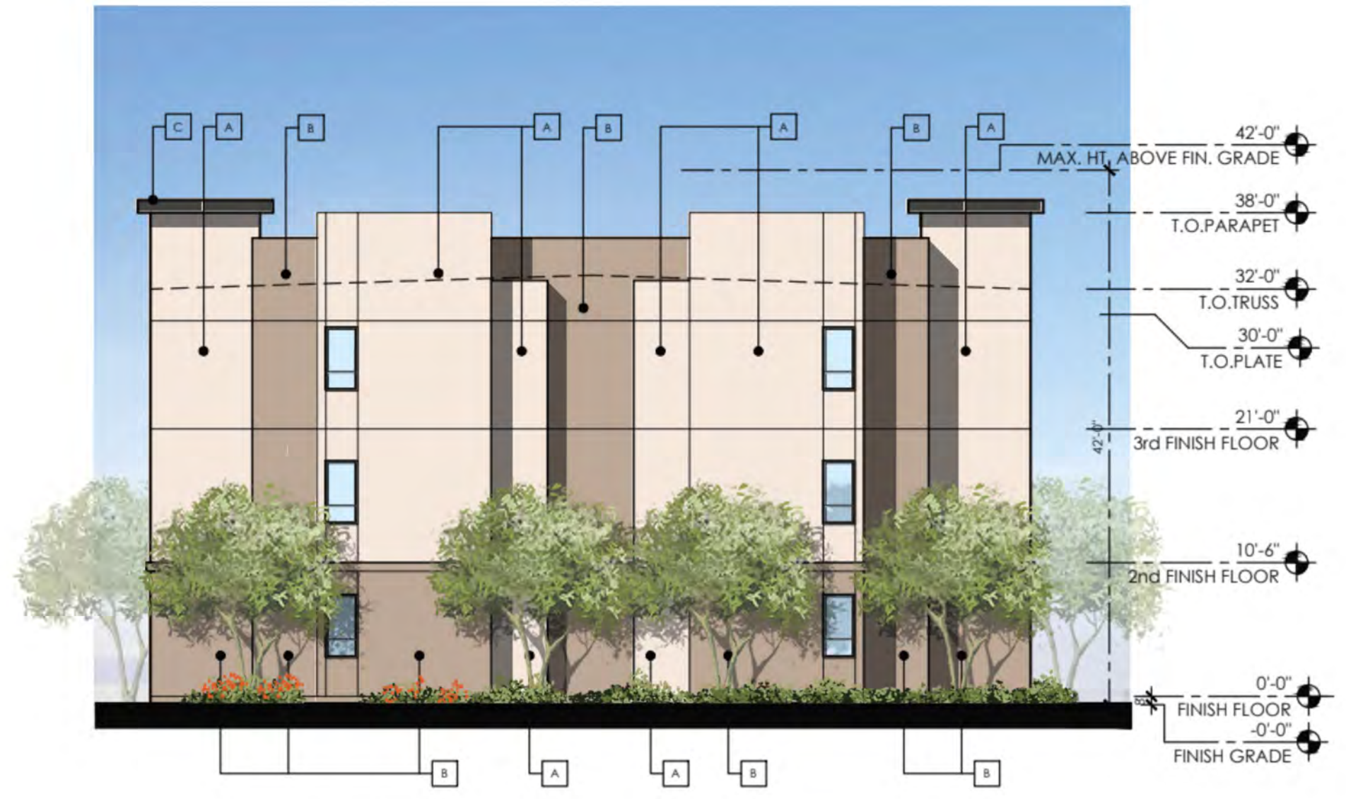
BUILDING TYPE 1A LEFT ELEVATION
