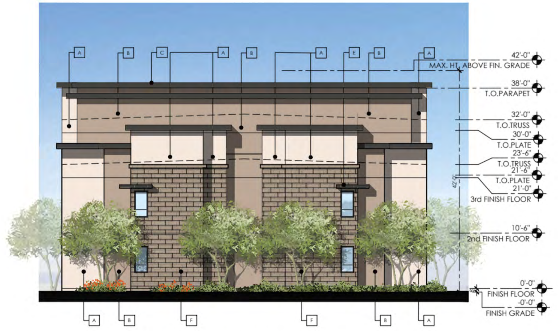
BUILDING TYPE 1C LEFT ELEVATION
