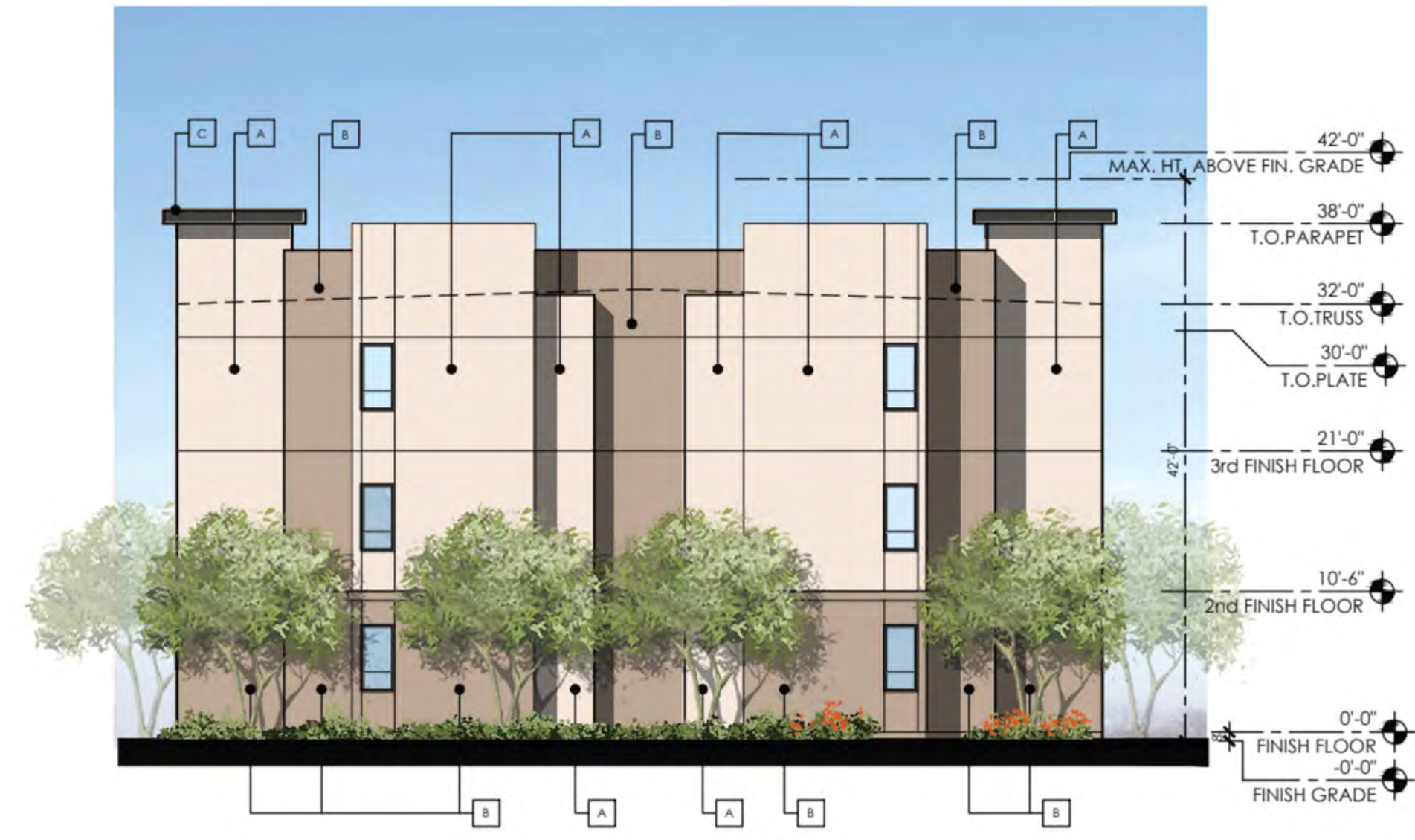
BUILDING TYPE 1A RIGHT ELEVATION
