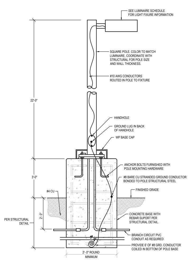
NOTE: THE POLE MANUFACTURER SHALL PROVIDE AN ENGINEERED POLE BASE DESIGN FOR 100 MPH WIND LOADING WITH A 1.3 GUST FACTOR. THE POLE BASE DESIGN SHALL BE FROM A STRUCTURAL ENGINEER REGISTERED IN THE STATE OF ARIZONA. THE STRUCTURAL ENGINEER SHALL VERIFY THE WIND LOADING AND GUST FACTOR CRITERIA ABOVE ARE ADEQUATE FOR THE AREA OF INSTALLATION.
